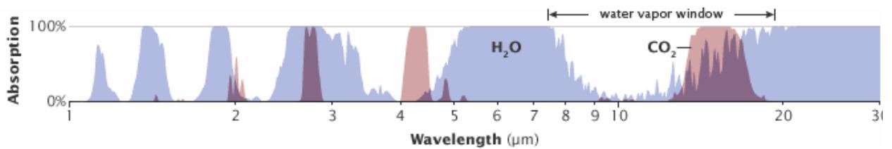
Figure 3: Absorption spectra of water vapour and carbon dioxide (3)
