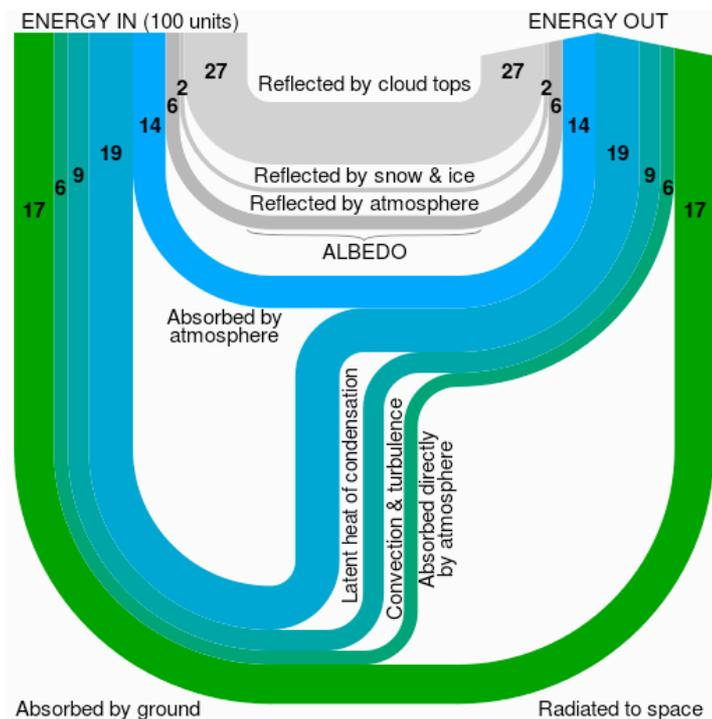
Figure 7: Earth heat balance – Sankey diagram (3)
